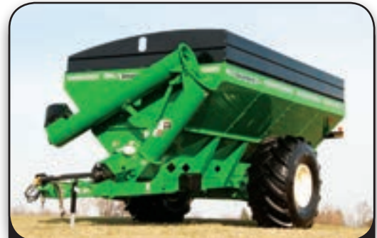
Upper portion of vertical unloading auger on both models rests on handy stand for quick return to the working position
